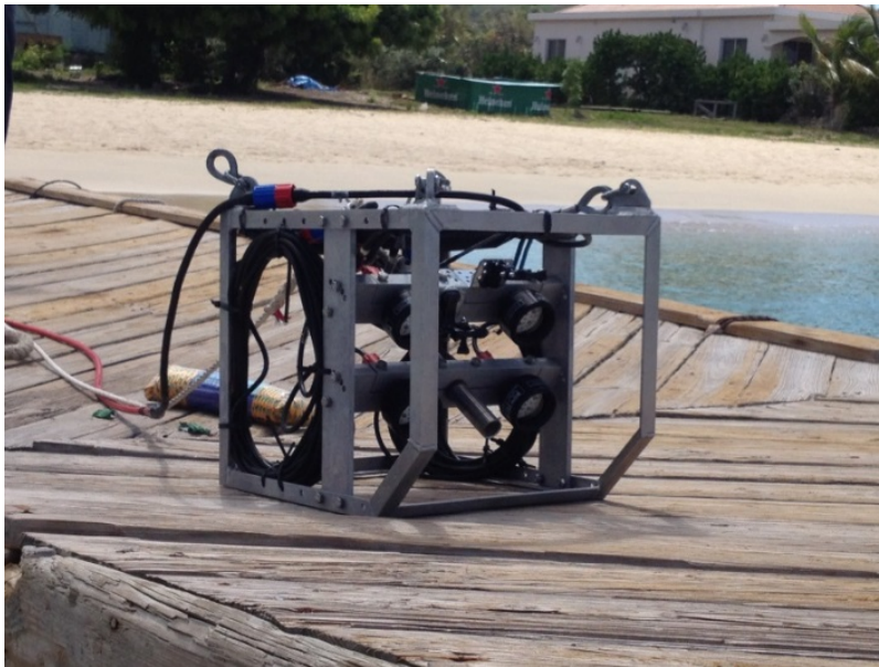
Figure 1: Aluminium underwater video array with lights, Bowtek live recordable feed camera and GoPro mounts for HD stills and video (source: DFMR archives).
